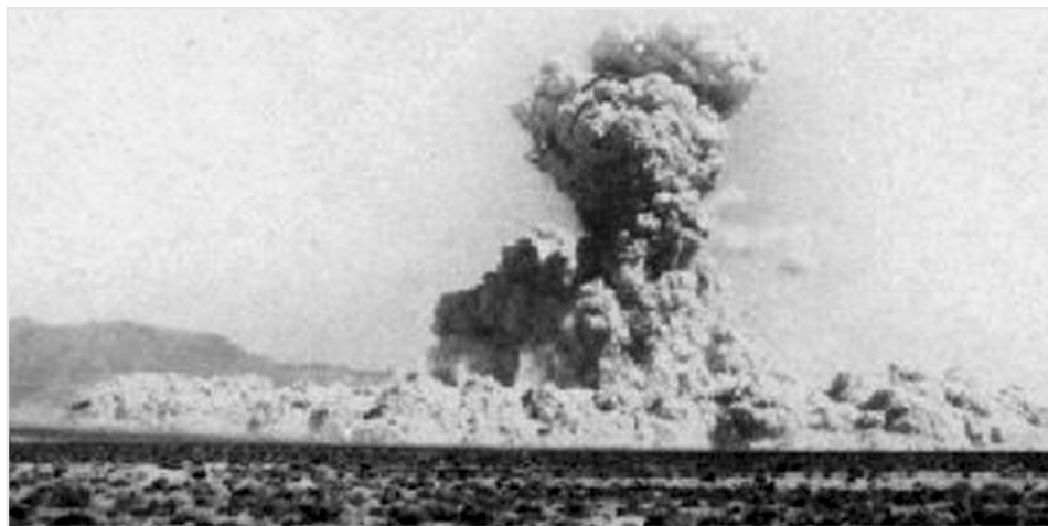
Figure 4. The 100 KT Sedan nuclear explosion, one of the Plowshares excavation tests, was buried at a depth of 635 feet. The main cloud and base surge are typical of shallow-buried nuclear explosions. The cloud is highly contaminated with radioactive dust particles and produces an intense local fallout.
