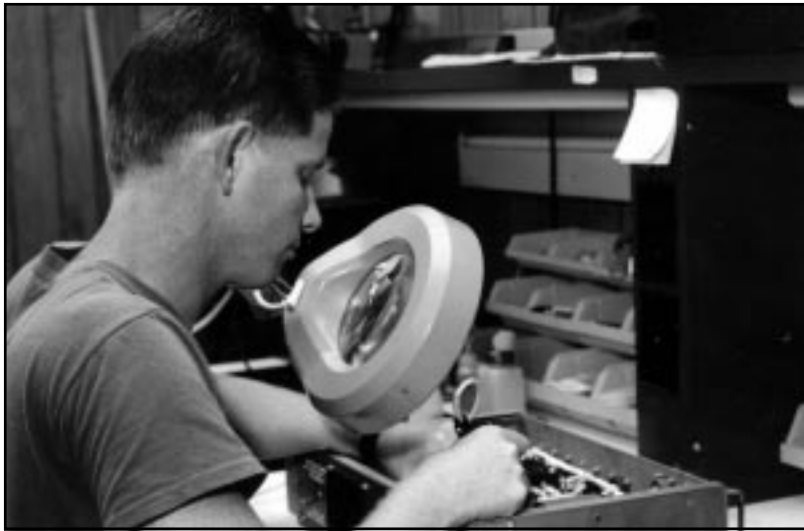
This airman uses an illuminated magnifying glass while performing maintenance of communications equipment.
