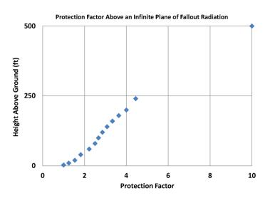
Figure C-2. Increase of PF with height over ground uniformly contaminated with fallout. Data do not include added protection provided by building materials.
