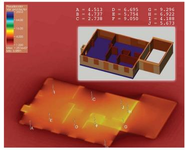
Figure C-7. PF calculation results for the first floor of a 2 story, brick sided home.
