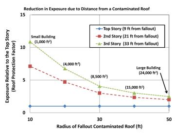
Figure C-4. PFs increase with distance from a contaminated roof.
