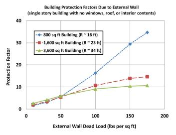
Figure C-5. PFs increase with the exterior wall mass (dead load).
