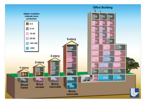
Figure 26. Example protection factors (PFs) for a variety of building types and locations. Adapted from (Ferlic, 1983) and (DCPA, 1973).
