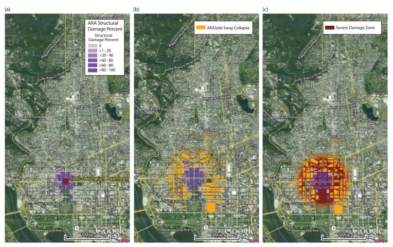
Figure A-3. (a) Structural damage, (b) potential side-sway collapse buildings, and (c) extent of the SDZ for the downtown Washington, DC scenario.
