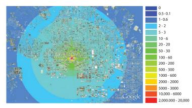
Figure A-9. Ground overpressures in psi modeled by NucFast for the illustrative Washington, DC scenario.
