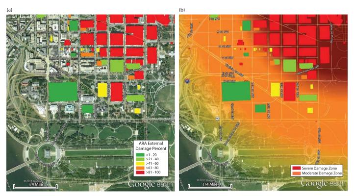
Figure A-8. Figure A-8. (a) Predicted area of external wall damage and the (b) MDZ for the illustrative scenario.
