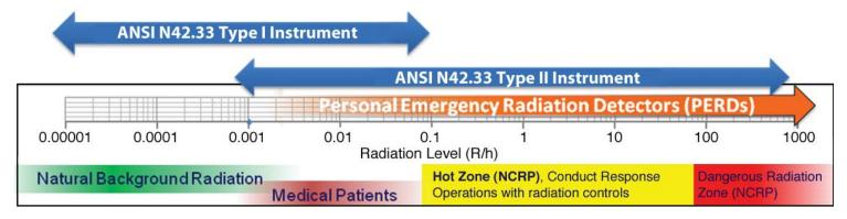
Figure D-2. Applicable exposure rate ranges for selected instrument types.
