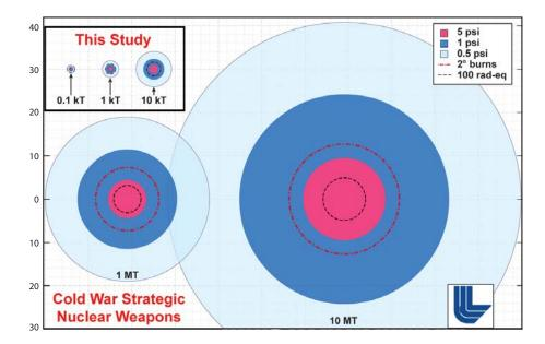
Figure 1. The different colors and lines identify damaging pressures, burns, and doses associated with detonations of various size. The present report is concerned with low-yield nuclear weapons that are far smaller in scale that those associated with the Cold War.
