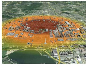
Figure A-7. The MDZ for the downtown Washington, DC scenario is represented by the orange area (some buildings are removed in the image to highlight the area of collapse).
