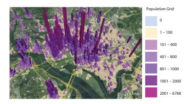
Figure 2. The finer of two modeling scales (100- by 100-m cells) is shown here for downtown Washington, DC to illustrate typical daytime population density. By incorporating other modeled information, each cell can also be used to display overpressures from a nuclear blast, thermal effects, prompt radiation, and fallout doses among other information.
