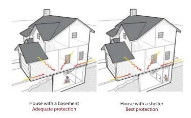
Figure 27. Protection can vary depending on location in a building. In this illustration, the best protected location is in the basement against an earthen wall.
