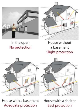
Figure C-12. Protection can vary depending on location in a building. In this illustration, the best protection is in the basement against an earthen wall. overall poor protection, select areas, such as a concrete-lined stairwell, might offer adequate protection.
