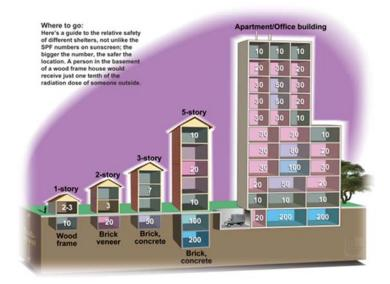
Figure C-1. Example PFs for a variety of building types and locations. Adapted from Ferlic (1983) and DCPA (1973).
