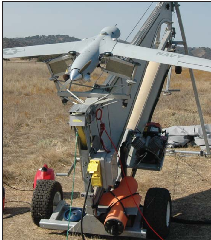
A Scan Eagle unmanned aerial vehicle sits on a launch sled during USSOCOM sponsored Tactical Network Topography 07-1 experiment at Camp Roberts, Calif.
