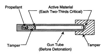
Figure 2-VII. Gun Assembly Principle
