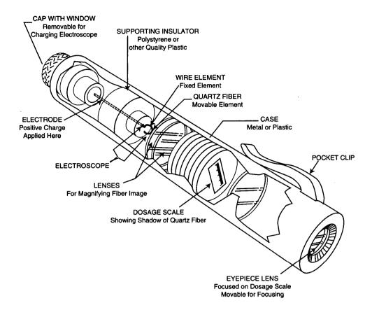
Figure A-I. Pocket Dosimeter
