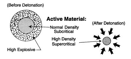
Figure 2-VIII. Implosion Assembly Principle
