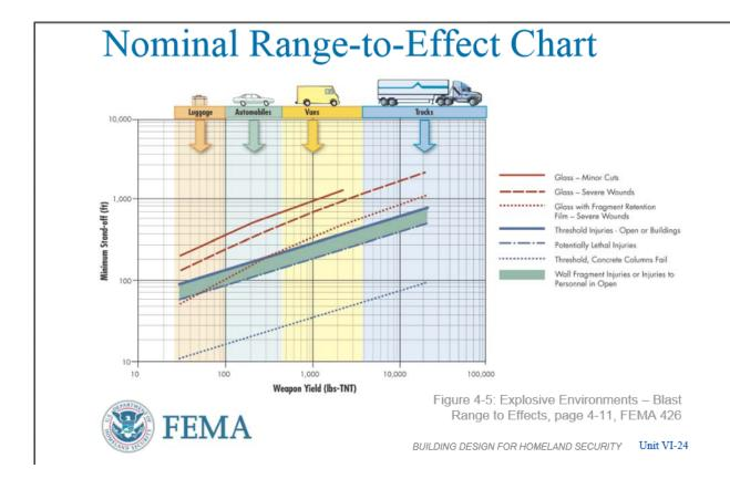
FEMA chart showing that the cutoff of damage from a tractor-trailer loaded with explosives is at about 2500 feet.
