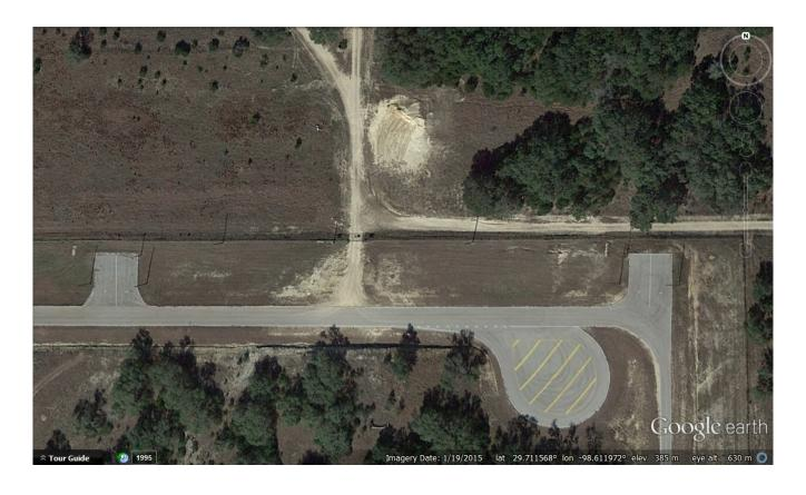
Appearance of facility, 2015. The large circle is a typical provision for turning long vehicles. The poles adjacent to the rectangular parking areas are possibly for lightning protection.
