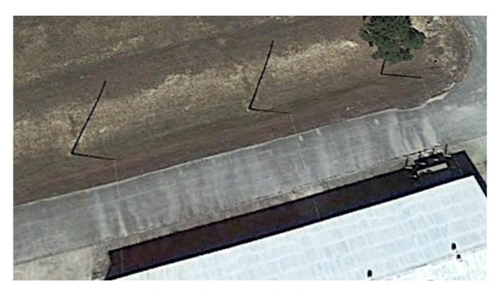
Close-up of masts on north side of building. Faint lines, possibly overhead ground wires, extend from the masts toward the building.
