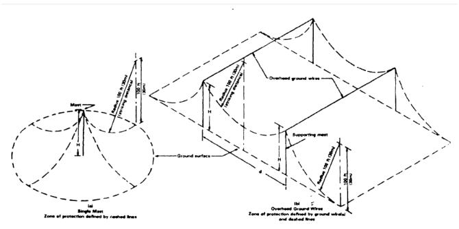
Figure 1 - Zone of Protection for Mast Height "H" Exceeding 50 Feet (15m)
