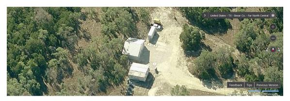
The largest structure, built in 2003, appears to be set into a notch cut into a steep slope with retaining walls toward the back of the building. The function of the five square pads in front of it is unknown.
