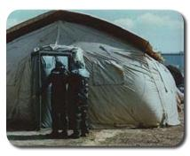
The M28 CPE is a low cost method of transforming existing tentage into an NBC collective protection shelter for command, control and communication
