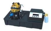
The Joint Service Mask Leakage Tester (JSMLT) is a portable test system capable of testing the serviceability of a protective mask in the field. It has expanded capability compared to the M41 PATS by allowing component level testing of the mask as well as system level testing with added components. It provides capability for an overall mask serviceability and fit factor validation of protective masks in the field.
