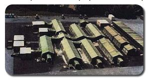
The Army's CP DEPMEDS program is a Joint effort to insert environmentally controlled collective protection into currently fielded hospital shelters. The requirement is to be able to sustain medical operations for 72 hours in a chemical contaminated environment. Environmentally controlled collective protection is
