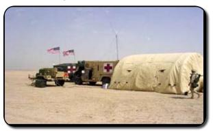
CBPS is a highly mobile, rapidly deployable shelter system designed to be used for Level I and II forward area medical treatment facilities and forward surgical teams. CBPS also replaces the M51. The CBPS consists of a dedicated M1113 Expanded Capacity Vehicle (ECV), a Lightweight Multipurpose Shelter (LMS) mounted onto the vehicle, a 300 square foot airbeam supported CB protected shelter, and a High Mobility Trailer with a towed 10kw Tactical Quiet Gen-
