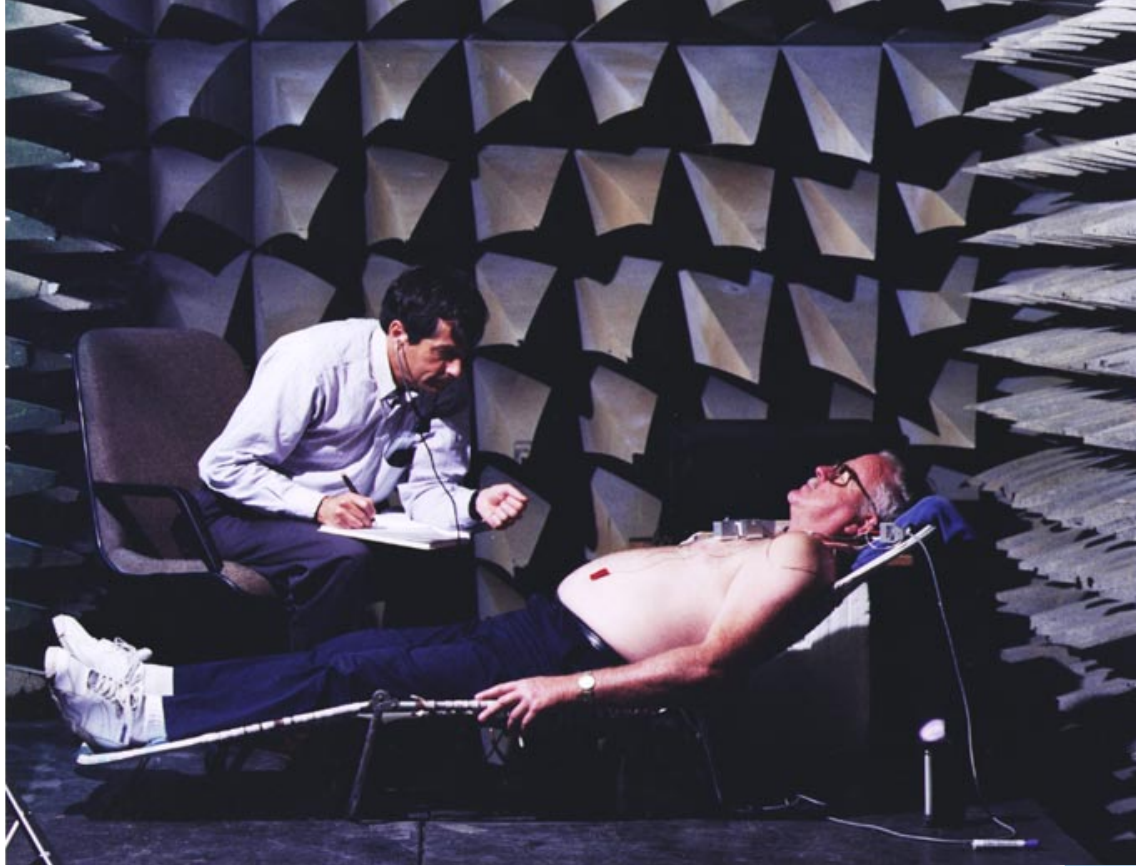
Coronary testing in the Anechoic Chamber
