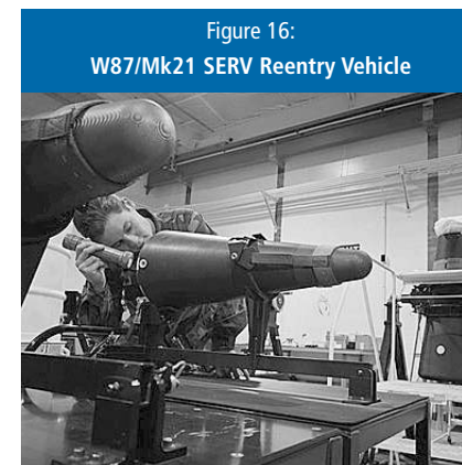
A U.S. Air Force technician inspects the fuze section on an Mk21 SERV reentry vehicle for the W87 warhead. Under a minimal deterrence posture, the secondary on this 300-kt warhead is not needed.
