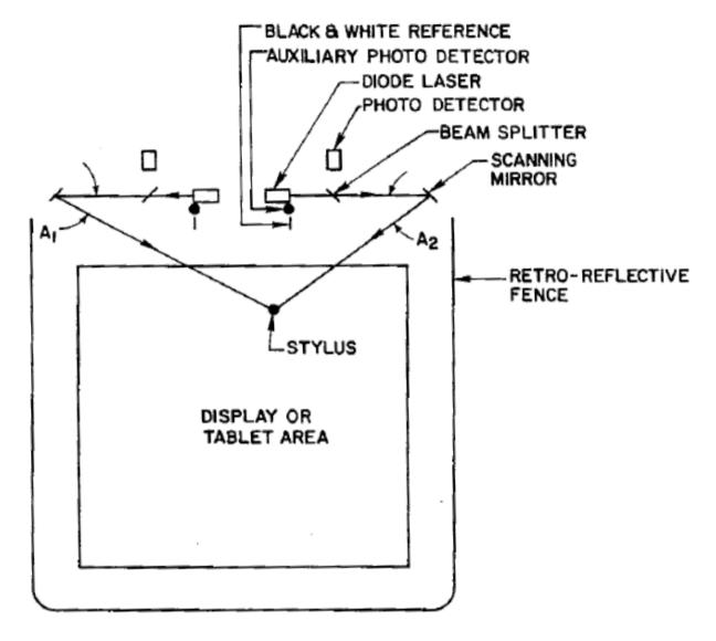
FIGURE 1: Device geometry and parts arrangement.
