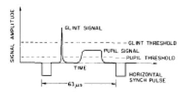
Fig. 5. Video signal for a raster line which crosses the glint and then the pupil. Typical threshold levels are indicated (dashed lines) as well as the horizontal synch pulses.
