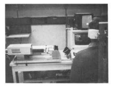
Fig. 4. Photograph of the eyetracker. The illumination system is inside the white tube in the background. The TV camera is at the left. The gimballed aiming mirror is just to the left of the display terminal.
