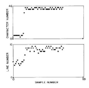
Fig. 11. Tracking record. A target was moved from screen location (5,5) to location (39,9). The sampling interval was 20 ms.
