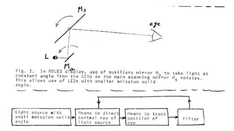
Fig. 3. Block diagram of display using servoed exit pupil.
