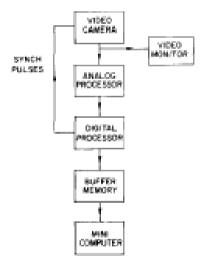
Fig. 6. Block diagram of the signal processing system.
