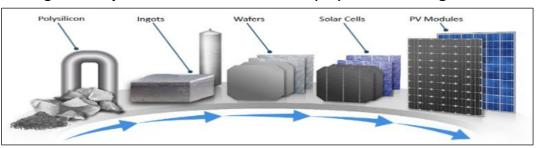
Figure I. Crystalline-Silicon Photovoltaic (PV) Manufacturing Process
