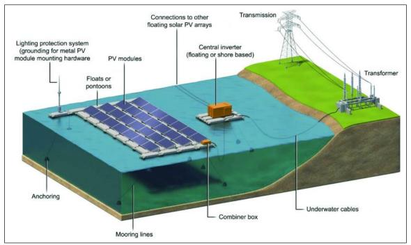
Figure 8. Diagram of a Floating Solar Photovoltaic System
