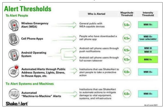
Figure 9. Alert Communication Pathways and Minimum Thresholds
