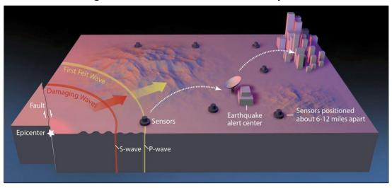
Figure 5. Schematic of the ShakeAlert System
