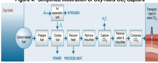
Figure 4. Simplified Illustration of Oxy-fuels CO<sub>2</sub> Capture
