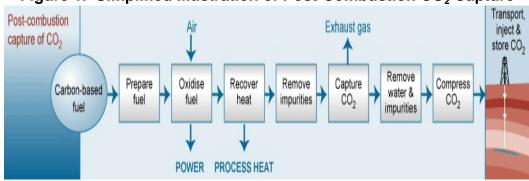
Figure 1. Simplified Illustration of Post-Combustion CO<sub>2</sub> Capture
