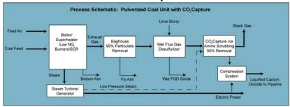
Figure 11. Representative Pulverized Coal Plant: Gavin Plant (Ohio)
