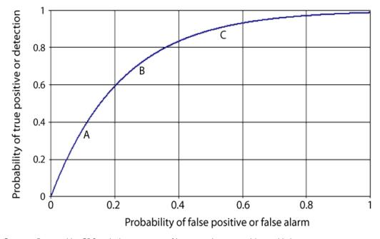
Figure 7.A Notional Receiver Operating Characteristic (ROC) Curve
