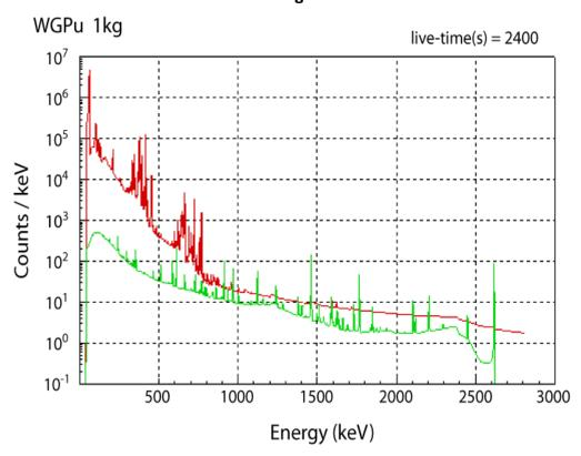
Figure 2. Gamma-Ray Spectra: Weapons-Grade Plutonium vs. Background
