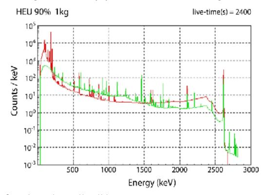
Figure I. Gamma-Ray Spectra: 90% Uranium-235 vs. Background
