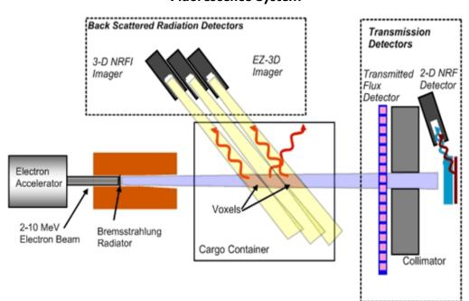
Figure 18. Schematic Diagram of Nuclear Resonance Fluorescence System
