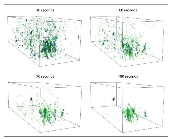
Figure 16. Muon Tomography Resolution Increases with Scan Time
