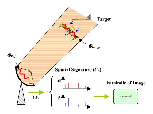
**Figure 14.** Field imaging – spatial signature discrimination. Field imaging may be a useful tool to aid or enhance RADAR/LIDAR target classification and identification. Real-time configurable spatial reference functions permit the synthesis of adaptive spatial filters and/or optimal detection algorithms.
