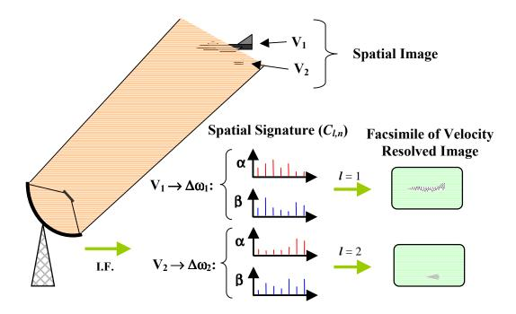
**Figure 15.** Doppler imaging – velocity field discrimination. Spatially distinguishable targets may be velocity resolved through the (temporal) frequency filtering of Doppler shifted spatial Fourier coefficients,  $C_{l,n}$ . *l* is the Doppler shifted index representing the *l*<sup>th</sup> I.F. bandpass frequency,  $\Delta \omega_i$ , (see **Equations 13-14**).
