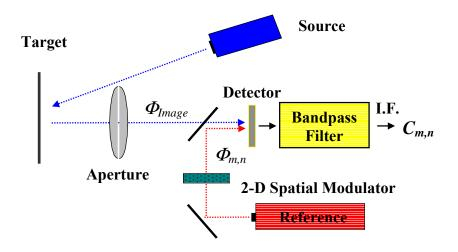
**Figure 3.** Fourier transform heterodyne field imaging. Based on coherent detection principles, FTH applies Fourier projection concepts through the transverse spatial encoding ( $\Phi_{m,n}$ ) of the local oscillator for electromagnetic field capture. FTH preserves both spatial amplitude and phase information.
