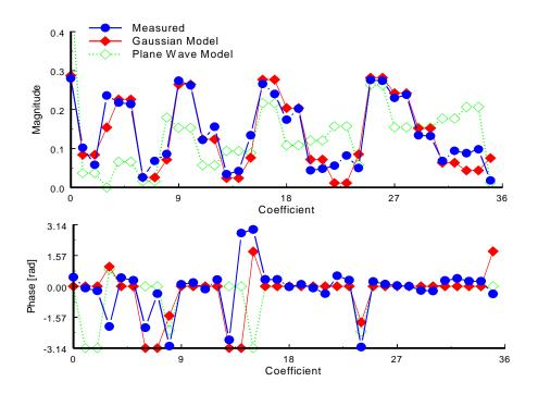
**Figure 8.** Measured spectral coefficients for no target. Included are plane-wave and Gaussian ( $\omega = \frac{1}{2}$ ) coefficients for baseline comparison (coefficients have been normalized) with Gaussian model providing the best fit.
