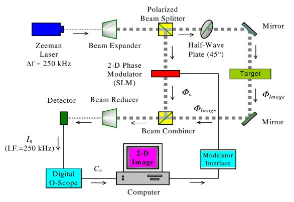
Figure 4. Schematic diagram of FTH experiment.
