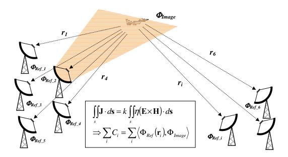
**Figure 17.** Coherently phased sparse-array. Coherently phased sparse arrays for improved spatial resolution and detection of low cross-section targets. Receivers phasing ( $\Phi_{Ref}$ ) is accomplished through addition or subtraction of phase pedestal offsets at the receiver local oscillator and delay offsets to the  $C_i$  before summation.
