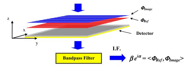
**Figure 2**. Heterodyned square-law detection can be perceived as a Fourier projection with the intermediate frequency (I.F.) current conveying the magnitude ( $\beta$ ) and phase ( $\alpha$ ) of the projection.
