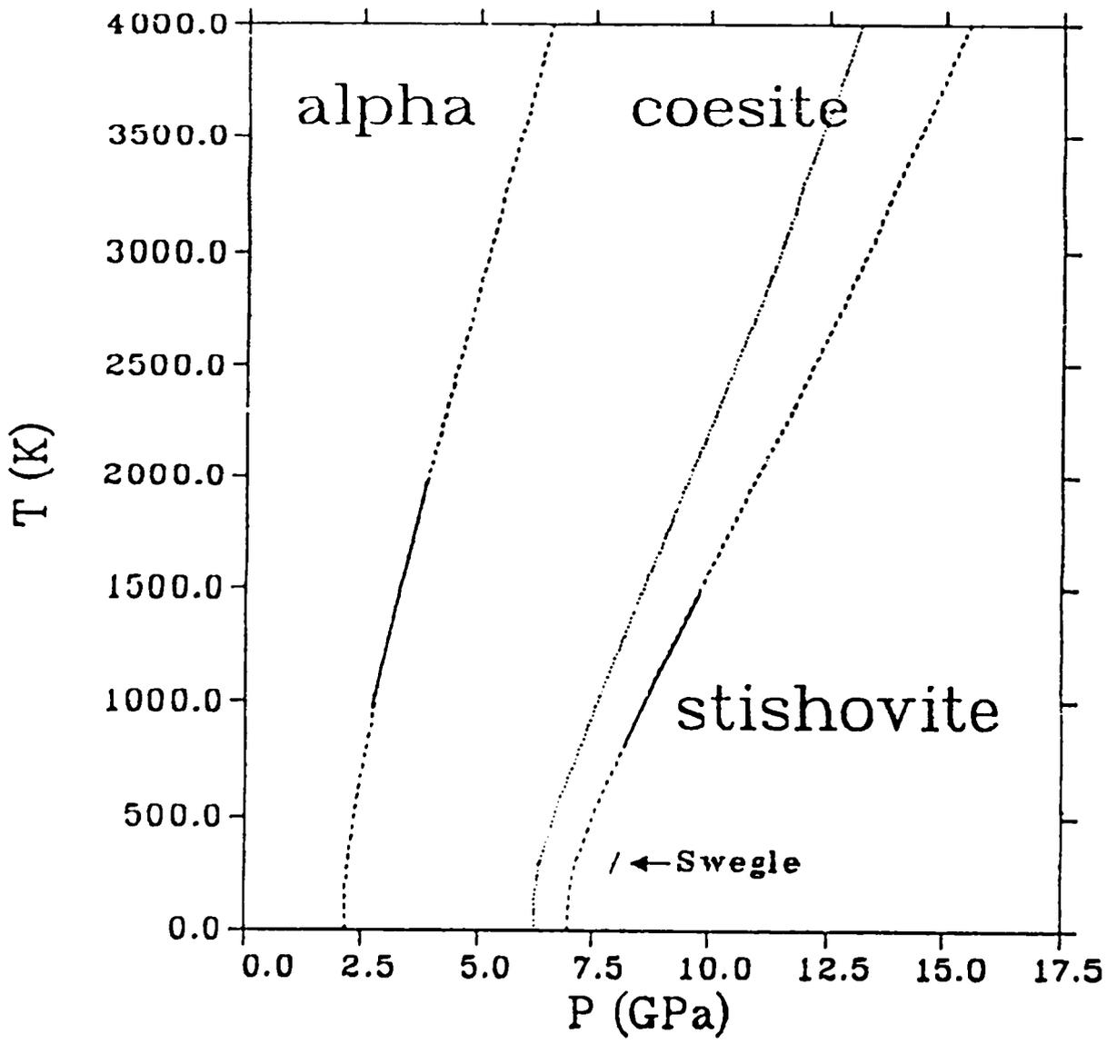
Fig. 1. The theoretical phase diagram for  $\text{SiO}_2$  (dashed lines) compared with the experimental alpha  $\rightarrow$  coesite (Ref. 10) and coesite  $\rightarrow$  stishovite (Ref. 11) boundaries (solid lines). Also shown are the hypothetical alpha  $\rightarrow$  stishovite boundary obtained here (dotted line) and that used by Swegle (Ref. 1).
