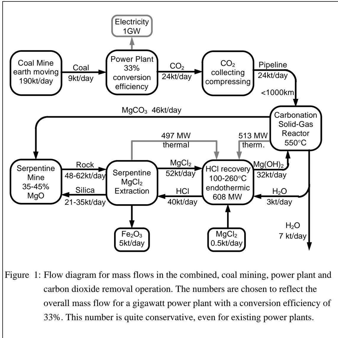
Figure 1: Flow diagram for mass flows in the combined, coal mining, power plant and carbon dioxide removal operation. The numbers are chosen to reflect the overall mass flow for a gigawatt power plant with a conversion efficiency of 33%. This number is quite conservative, even for existing power plants.
