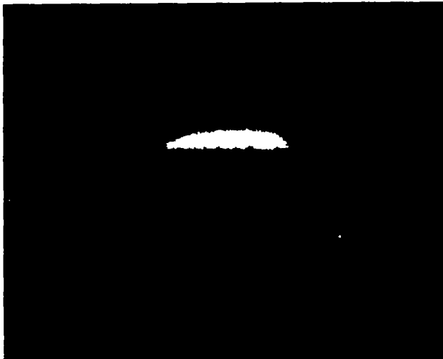
Fig. 7. An edge view of the tritium source in one atm of neon obtained during a 1/30-sec exposure. A 2-1/2-in.-diam f/0.85 lens and an RCA 8606 image intensifier were used in conjunction with a Polaroid scope camera and 3000-speed film to obtain this photograph.
