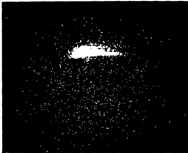
Fig. 8. An edge view of the tritium source in one atm of deuterium obtained during a 10-sec exposure. A 2-1/2-in.-diam f/0.85 lens and an RCA 8606 image intensifier were used in conjunction with a Polaroid scope camera and 3000-speed film to obtain this photograph. Notice the spots due to the large dark current and the range of the beta rays compared with those in Fig. 7.
