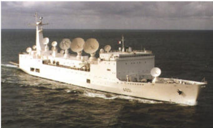
FIG 6: The French tracking ship "Monge", with its ARMOR tracking radars.
