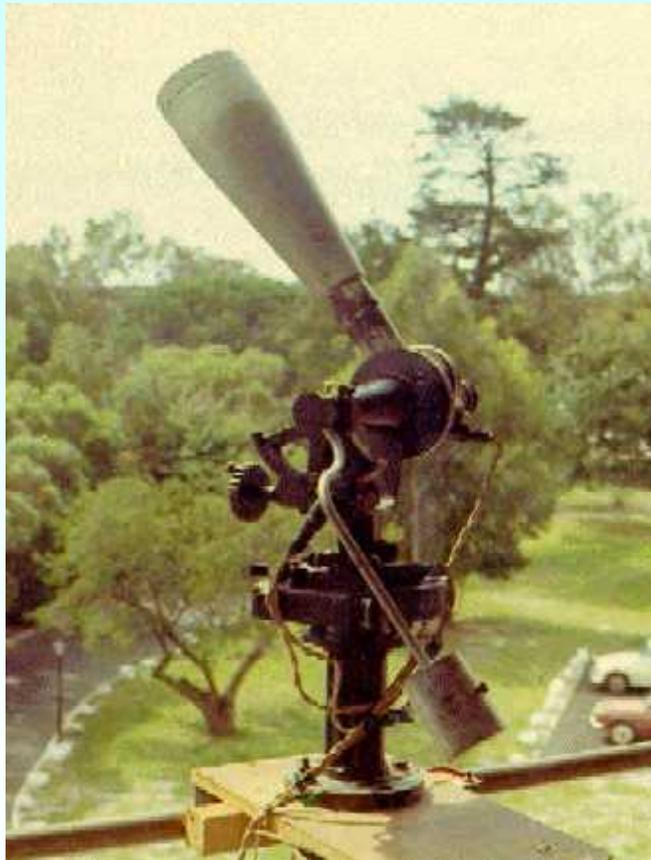
The original mount was used by the US military in WWII for aiming big naval guns. Around 1960 the mount was made available to the MOONWATCH network and carried a 5 inch f/5 refractor designed to be able to track the 6inch diameter Vanguard satellite at the highest point of its orbit.
