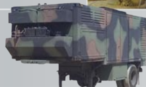
920kW Deployable Power Generation and Distribution System
