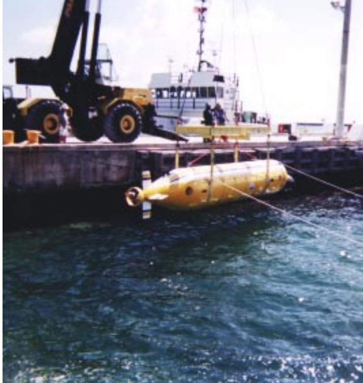
Perry Technologies' Mobile Undersea Systems Test UUV with two types of fiber optic tethers
