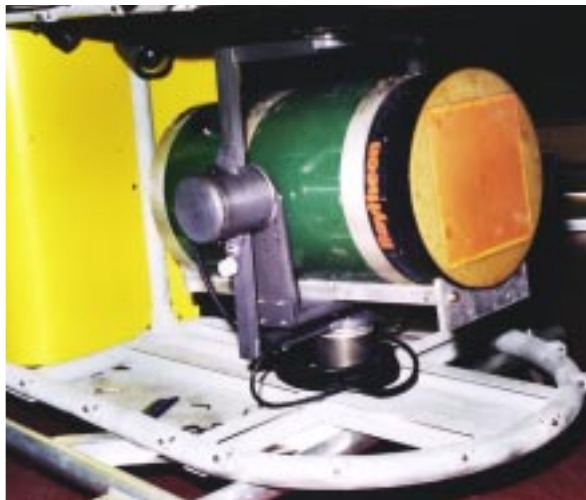
High resolution sonar array mounted on Towed Data Acquisition System (TDAS) (above)
