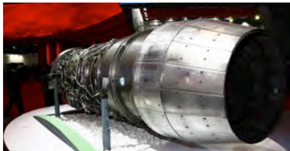
China's domestically produced WS-10 family of military turbofan engines, which power the J11-B, carrier-based J-15, and J-16 fighters.
