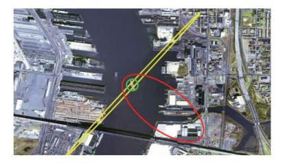
Real-world geolocation analysis on the test bench: the OPS simulation provides geolocation accuracy estimates for RF receiver / intercept systems against both radar and communications emitters.
