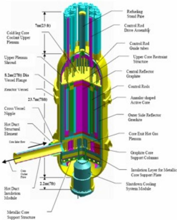
Fig. 2. Model of MHR design for high-temperature process heat applications.
