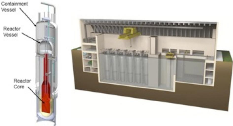
Fig. 4. Model of NuScale reactor and containment vessel (left) and plant (right).
