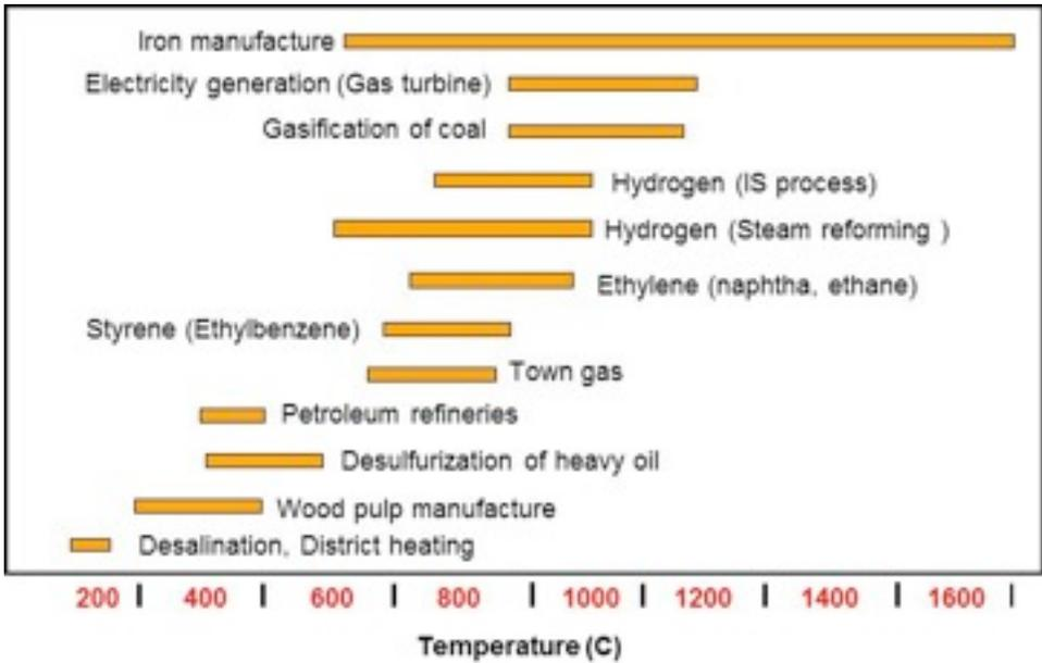
Fig. 1. Temperature requirements for various industrial processes<sup>123</sup>
