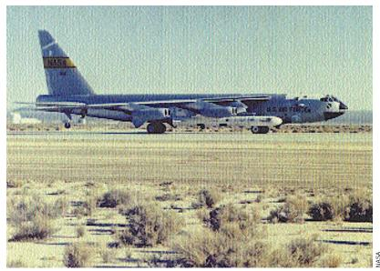
Pegasus air-launch space booster on board NASA B–52 carrier aircraft.
